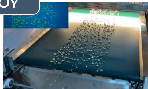
Nut sorting machine deploying perClass Mira models. Courtesy of VISRATEK
