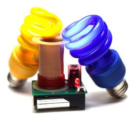
The Teslette works on the same principles as the Tesla coil and illuminates fluorescent bulbs using wireless energy transfer. This kit is easy to assemble and a great introduction to electronics.
