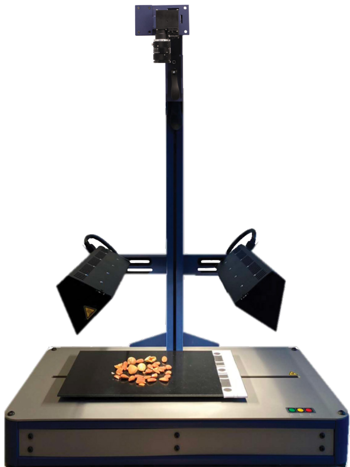
The Headwall MV.C VNIR hyperspectral imaging sensor mounted on the perClass Mira® Stage
