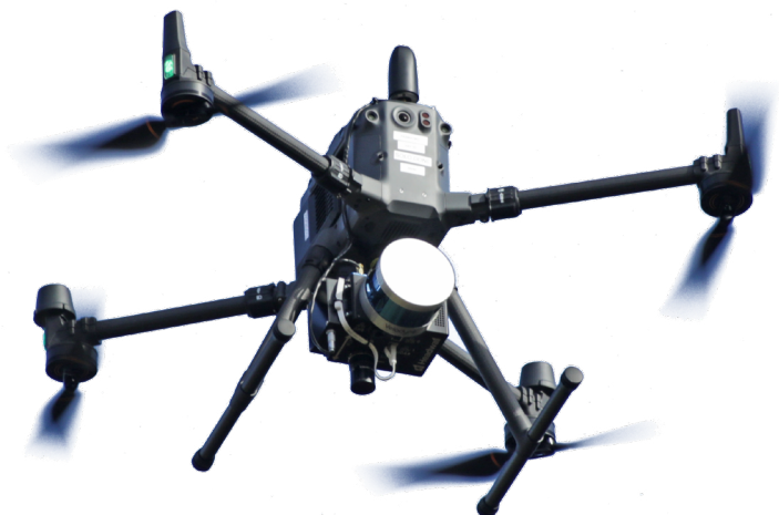
The Headwall Nano HP hyperspectral imaging sensor mounted on the DJI M350 drone, with LiDAR
